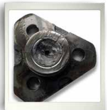
SPURIOUS AXLE PIVOT PIN
